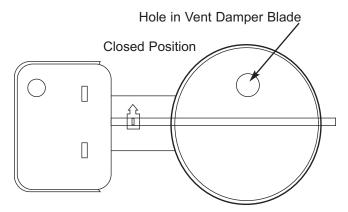
DO NOT plug the hole if installing the vent damper on a continuous pilot system as this will create a hazardous condition.
